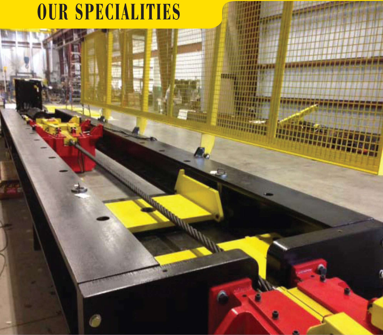
Computerised Load Test Machine (Test Bed) Load Testing Capacity: 150 Ton
